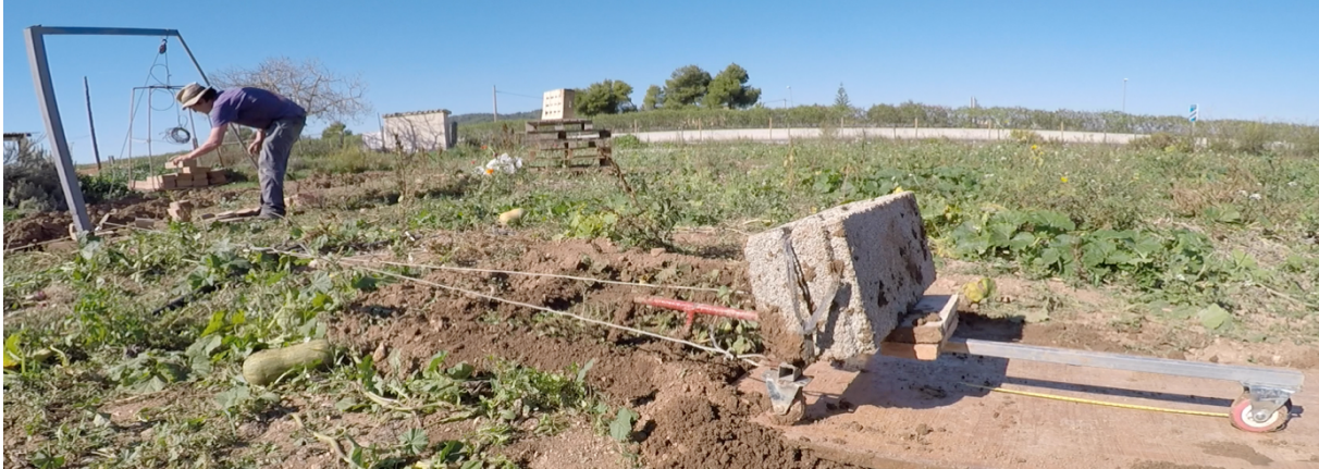
Figure 4: The actual experiment, here in a pumpkin field after harvest, in wet soil. The basket with bricks to the left is attached to a cable, which pulls the device on the right. Note the concrete block on top of the device, without which the device would rotate about the tip of the spike in the soil.
