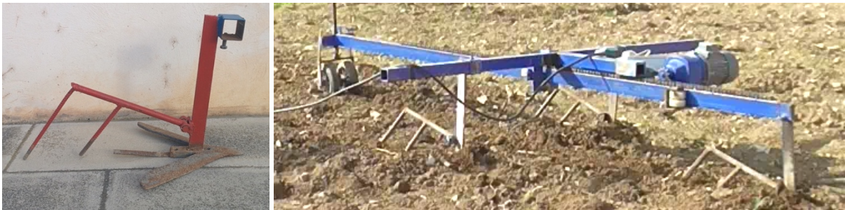
Figure 1. Left: Set of spikes with lever arm and movable joint, attached to the rear of a tillage tool. Right: Tillage device with one set of spikes and tillage tool in front of the main frame, and two sets of spikes and tillage tools on either side of the sliding frame. In the photo the device moves from left to right and the horizontal draft force acting on the spikes from the tillage tools is directed from right to left.
