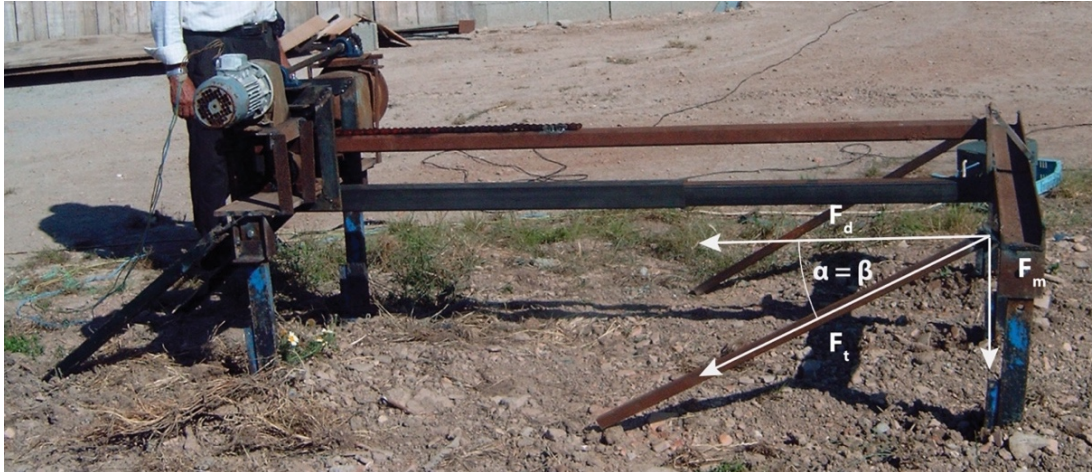
Figure 1: early design of interlocking spikes. The vehicle moves from left to right.
